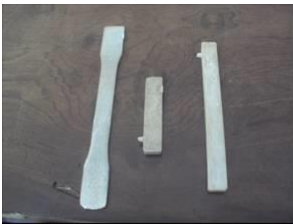
Figure 2. Samples produced by injection molding technique ready for testing (ASTM standards)
